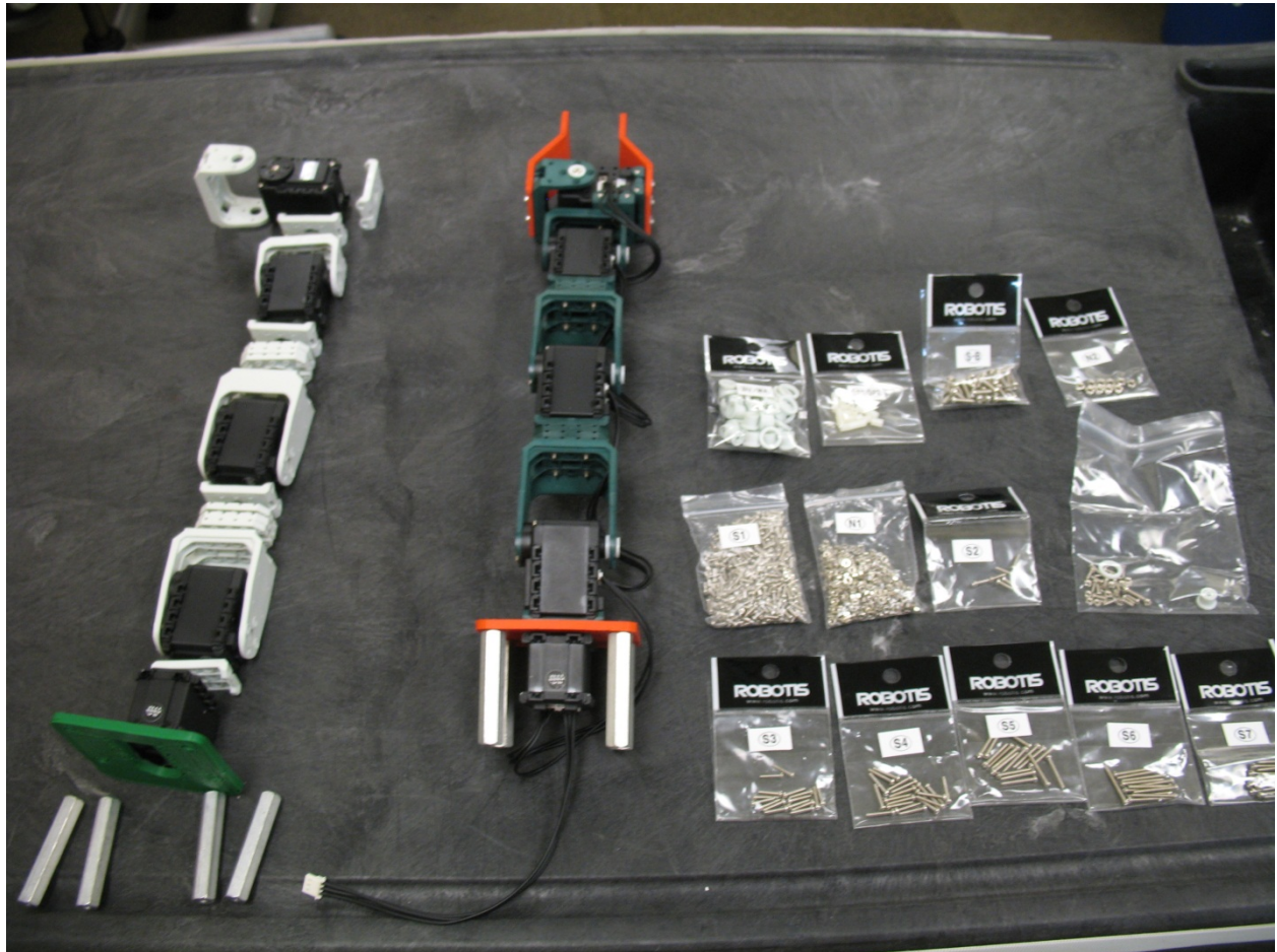
The unassembled arm components (left) and the assembled arm (right) along with associated Dynamixel accessories.
