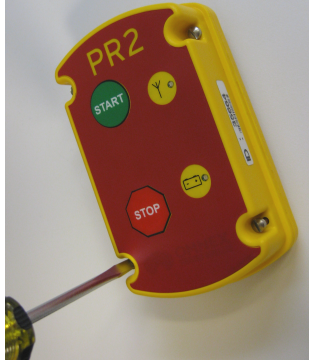
Figure 5.2: Opening the PR2 wireless run-stop to change the batteries.
